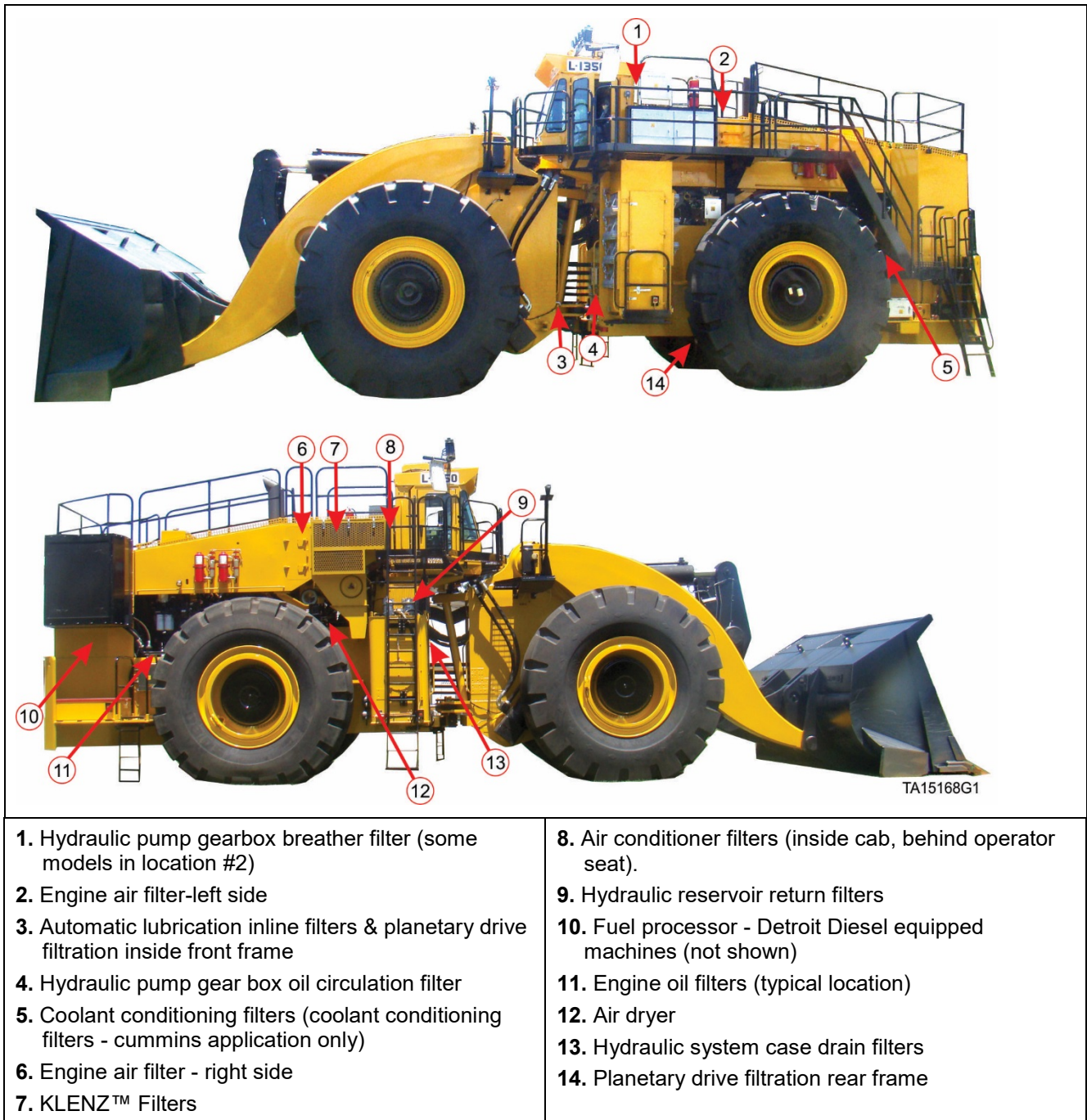
Figure 2. Filters – general machine locations (typical 1850/2350 machine)
